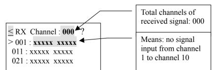
h line can indicate the values of 10 enamels in all. To browse the other values of inels, turn the multi-selector forward to select >, then press the multi-selector. At this time you can turn multi-selector backward or forward for this purpose.
