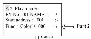
For some tests, first locate the > at the part [1] to select the desired function. Then locate the > at the part [2] to adjust the level by turning the multi-selector.
