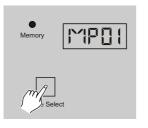
1. Tap Mode Select button until LED under Memory is lit, this unit is in Memory mode, the programs you made before will be activated in this mode.
