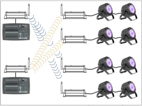
Rather than using fixed frequency channels, W-DMX<sup>TM</sup> technologie uses Adaptive Frequency Hopping technology to continually check the radio channels for interferences and to rapidly move operation to clear radio channels. The checks are carried out in combination with another advanced technology: time division multiple access. This technology makes the most efficient use of every visited frequency channel.
