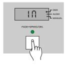
Tap the Fade+Speed button to receive record data, the Segment Display shows "IN".
