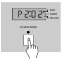
Create a scene on your DMX controller, tap the Record button to change the step(scene), all LEDs flash briefly indicating the old scene is replaced by the new one.
