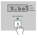
3. Tap the Fade+Speed button to change between "N-BO" and "Y-BO".
