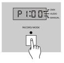
Press and hold down the Record/Mode button for five seconds, the LED above it lights indicating Record mode is active, the Segment Display shows the program and its scene of last time.
