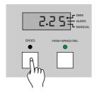
1. Tap the Speed or Fade+Speed button to select chase mode or fade mode, the LED above it lights indicating your selection.
