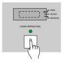
3. Tap the Fade+Speed button to send record data. During the period of sending, all other operation doesn't work.
