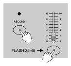
Press a Flash button between 25-48 while holding down the Record button. All LED will flash indicating the scenes have been programmed into memory.
