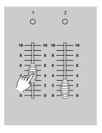
Create a desired scene using Channel Sliders 1-48. At 0% or DMX 0, these sliders should be at 0 position, and at 100% or DMX 255, these sliders should be at 10 position.
