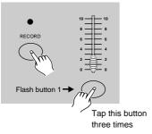
Tap the Flash button 1 three times while holding down the Record button, the Segment Display reads "CHI" indicating MIDI IN channel setup is available.
