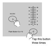
2. Tap the Flash button 5 or 10 three times while holding down the Record button.
