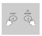
Tapping Flash 7 button three times while holding down Record button allows you to clear DMX channel setup and resume DMX channel to factory setting, i.e., 1-48 channel sequence.
