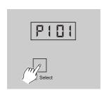
1. Pressing Prog. Select button three seconds activates Programming mode, the LED display shows "P" followed by three numbers. The second character indicates the program(1-7), and the last two characters indicate the step(01-16).
